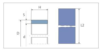
Calculating stretched length L2 for rods / pistons:  $L2 = (D-S) \times 3,11-0,5$  /  $L2 = (d+S) \times 3,11-0,5$
